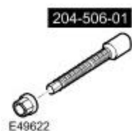
Halfshaft installer adapter 204-506-01
