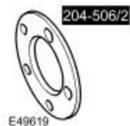
Halfshaft remover/replacer 204-506/2 (LRT-60-030/2)
