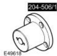
Halfshaft remover/replacer 204-506/1 (LRT-60-030/1)
